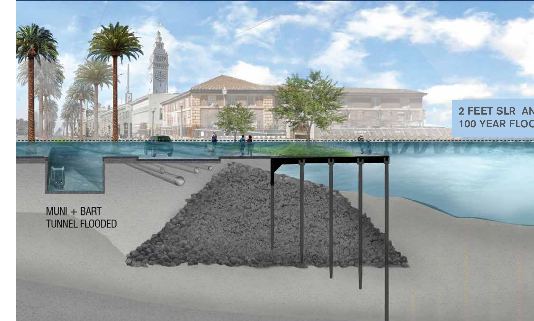
POTENTIAL FLOOD RISK TO MUNI AND BART TUNNEL AT RINCON PARK
