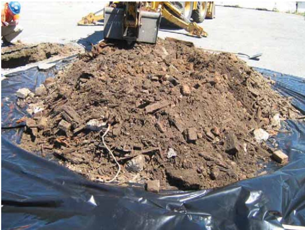
Photograph 6 - Bay fill material, Slipway Way Park SPTP-01
