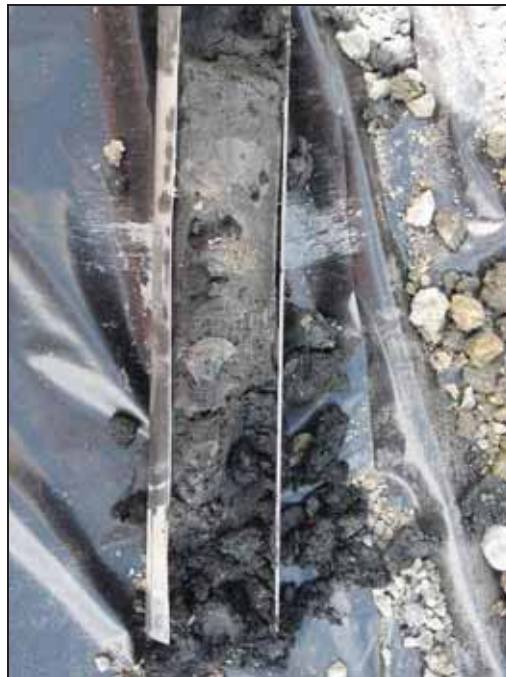
Photo 2: P2SB-02, 14-15 ft. marine deposit containing shell.
