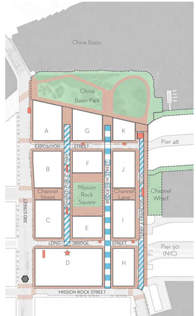
**FIGURE 2.3.1** Pedestrian Circulation + Accessibility diagram illustrating pedestrian routes and access, significant connections, and accessible loading zone locations in the public realm. See Chapters 3 and 4 for open space and street details.
