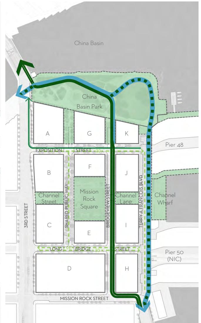
**FIGURE 2.4.2** Bicycle Circulation Network Diagram illustrating hierarchy and connections among the different types of bicycle facilities across the site. These facilities are described in Chapters 3 and 4 for each open space and street.
