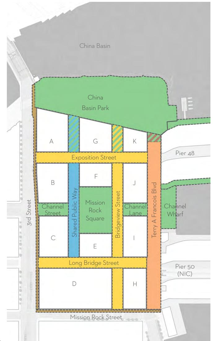
**FIGURE 2.2.1** Street Typologies diagram illustrating how the five street typologies defined in 2.2.1 are distributed across the site. These typologies are described in Chapter 4 in the controls for each street.
