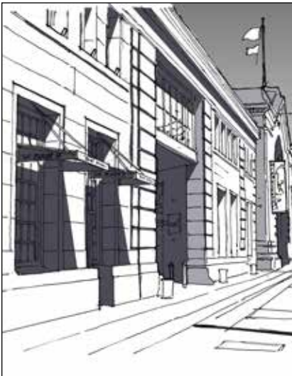
Fig. 32. Sketch of Awnings at ground-level Minor Windows.
