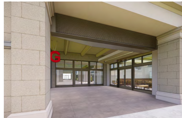
H LINEAR GRILLE ABOVE EXISTING OPENING
