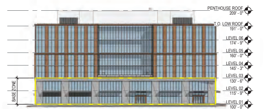
6 SOUTH ELEVATION BASE 1" = 40'-0"
