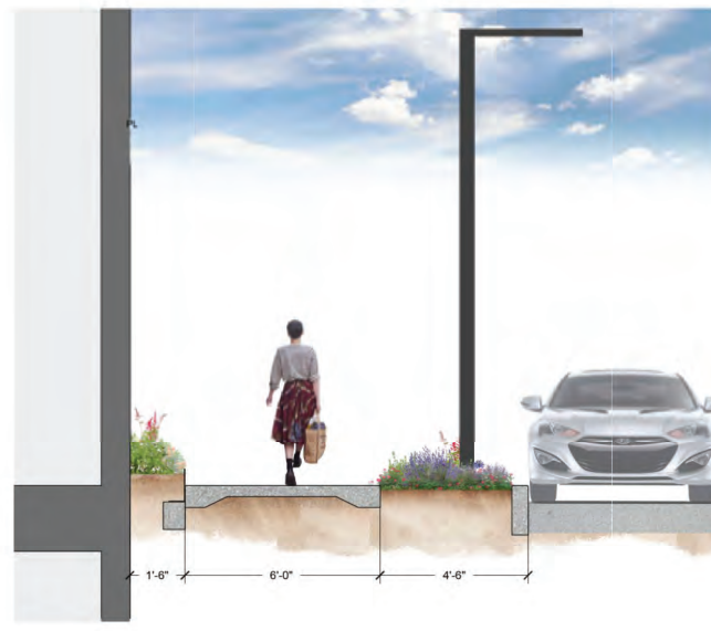
SECTION C - 20TH STREET SIDEWALK
