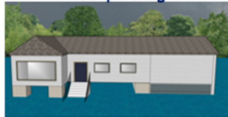
Raise structure in place
