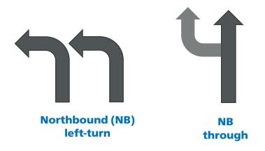
Restoring the two left-turn lanes and maintaining two northbound (NB) vehicle lanes on the far-side of the Broadway would likely improve conditions for all users - including drivers. While longer NB back-ups are expected, the 'green time' provided should help clear most vehicles each signal cycle; capacity for left-turns to Broadway meanwhile would be greatly improved.
