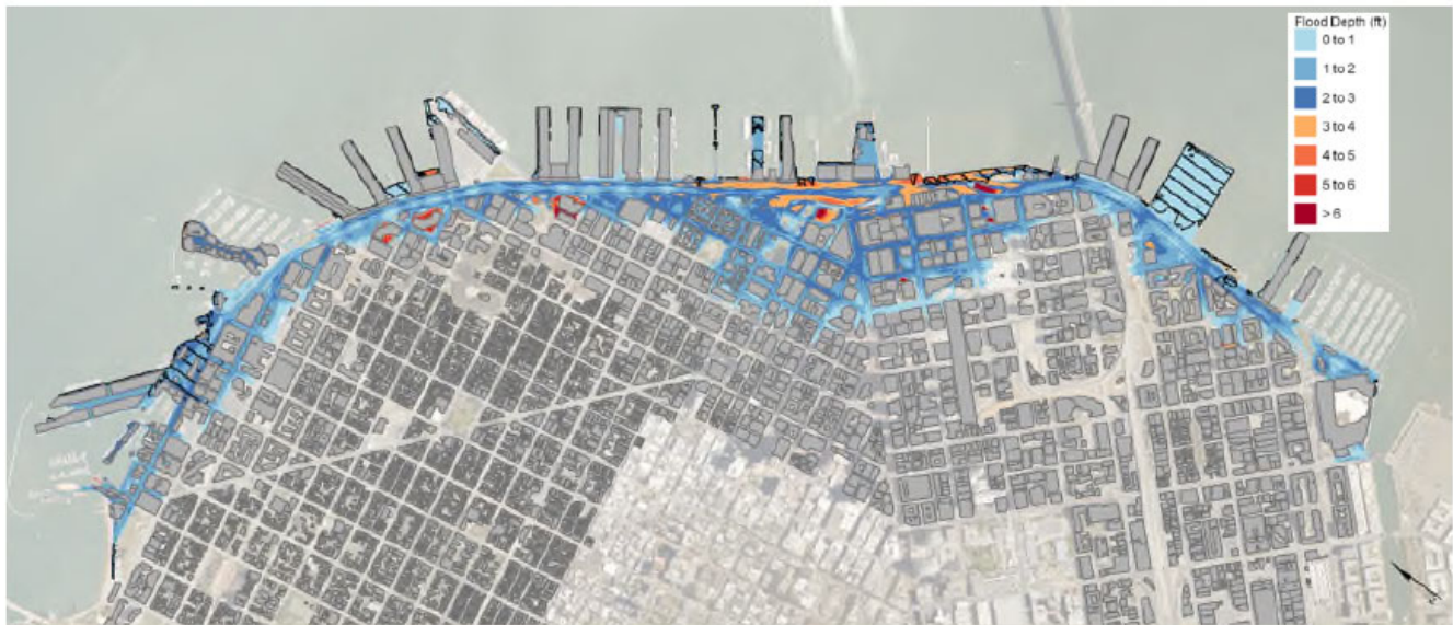
Figure 3-10. Inundation Map for 100-year Extreme Tide under 3.3 Feet of Sea-level Rise
