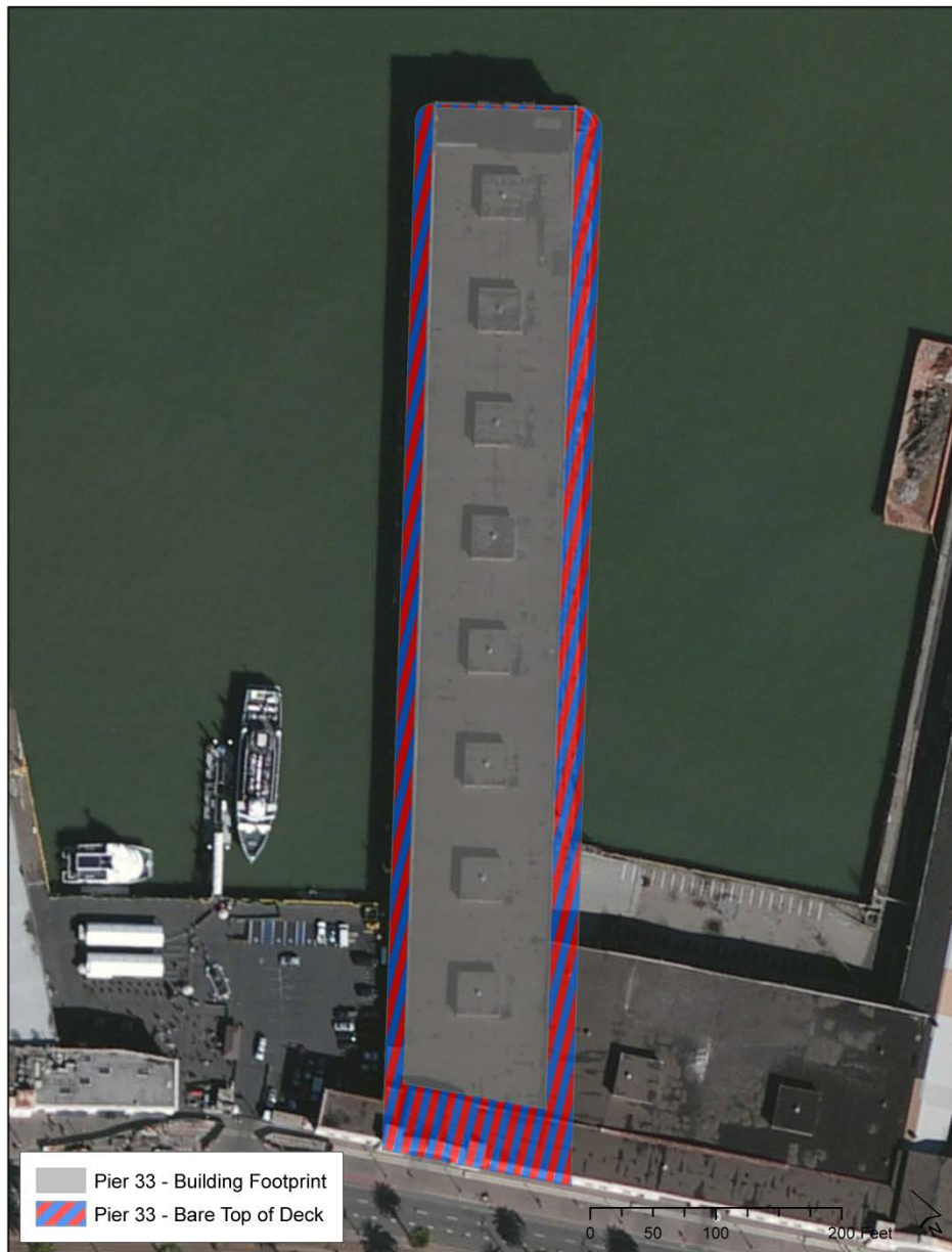
Figure 3-2: Example Area of Elevation Extraction at Pier 33
