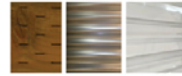
MAIN FENCE: PRESSURE TREATED WOOD POSTS, GALVANIZED STEEL PANELS, CORRUGATED TRANSLUCENT PANELS AT TOP
