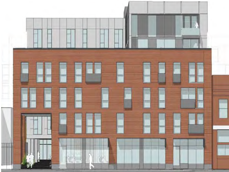
PROPOSED PROJECT JULIET BALCONIES DAVIS ST. ELEVATION
