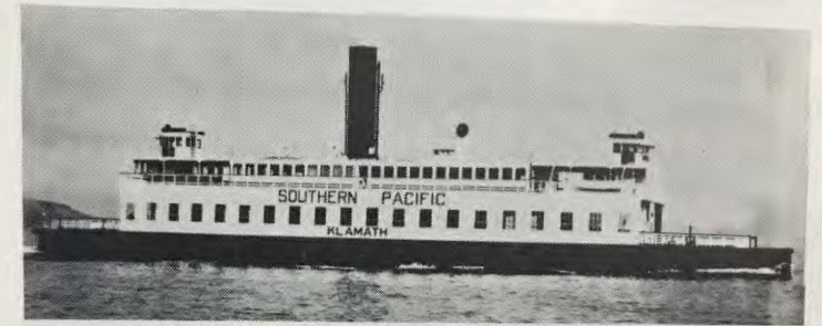
Klamath 224461 Screw Built 1925, Bethlehem Steel Co. Union Yard, San Francisco Operated by Southern Pacific, Southern Pacific-Golden Gate Ferries, Ltd., Richmond-San Rafael Ferry Steel hull, 234' x 45' x 17' 1952 tons Triple expansion engine, 19" x 32" x 56" x 36" 1400 hp Retired, 1956; rebuilt, 1964, as floating office and studio. Moored at Embarcadero, San Francisco
