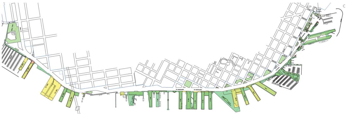
Figure 4: Structural condition rating map of substructures along the waterfront between Hyde Street Harbor and China Basin
