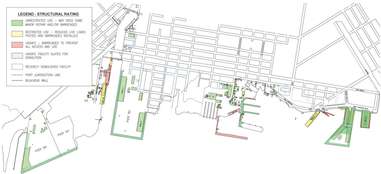
Figure 3: Structural condition rating map of substructures along the waterfront between China Basin and Pier 96
