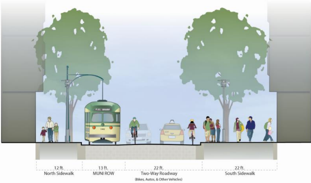
JEFFERSON STREET PROPOSED DESIGN TYPICAL STREET SECTION - LOOKING EAST FROM TAYLOR STREET
