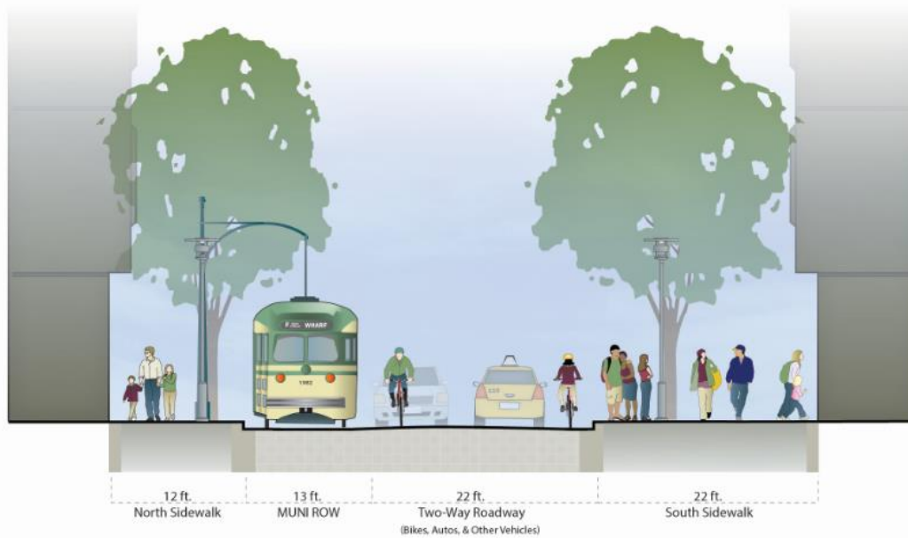
JEFFERSON STREET PROPOSED DESIGN TYPICAL STREET SECTION - LOOKING EAST FROM TAYLOR STREET
