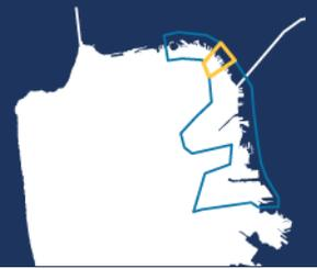
The primary flood pathways are from overtopping along the engineered shoreline. Flooding first occurs in this subarea due to floodwaters conveyed along the Embarcadero roadway that overtops the shoreline in Subarea 2-2. Higher Bay water levels eventually overtop the shoreline in this subarea, and floodwaters extend several streets inland.
