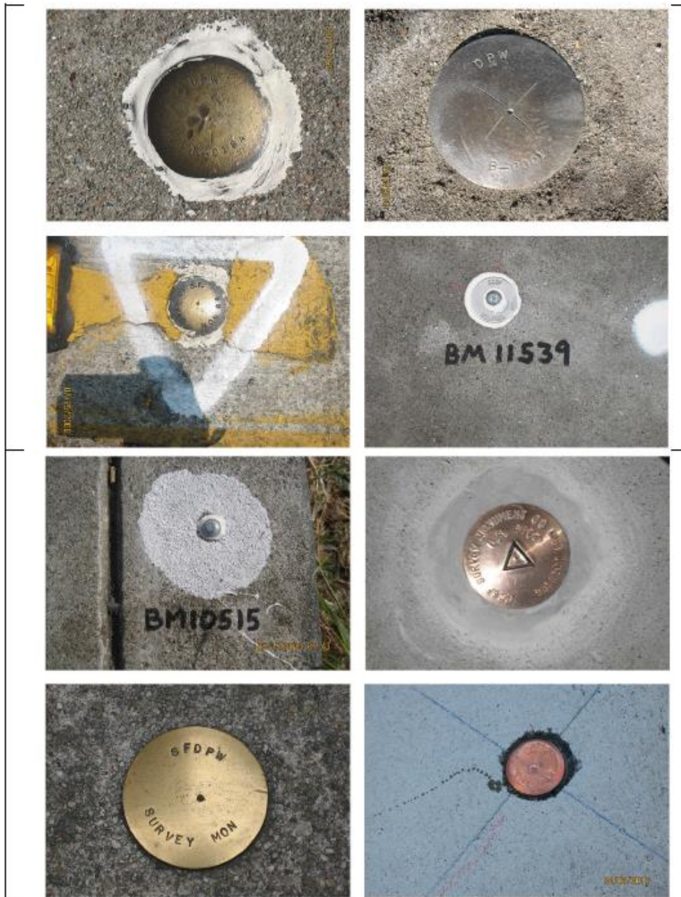
Figure 2 Typical Surface Monuments
