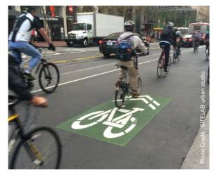
**FIGURE 4.5.2:** Example Class 3 Shared Lane (Sharrow) Pavement Marking
