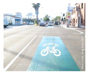
**FIGURE 4.5.3:** Example Class 3 Shared Lane (Super Sharrow) Pavement Marking
