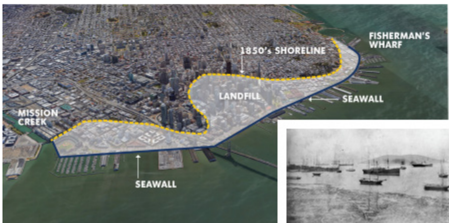
(ABOVE) The Seawall created over 500 acres of new land (RIGHT) The Seawall transformed what was once tidal mudflats along San Francisco's shoreline
