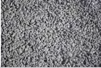
6a Alternative Bay Trail Paving: Porous Concrete
