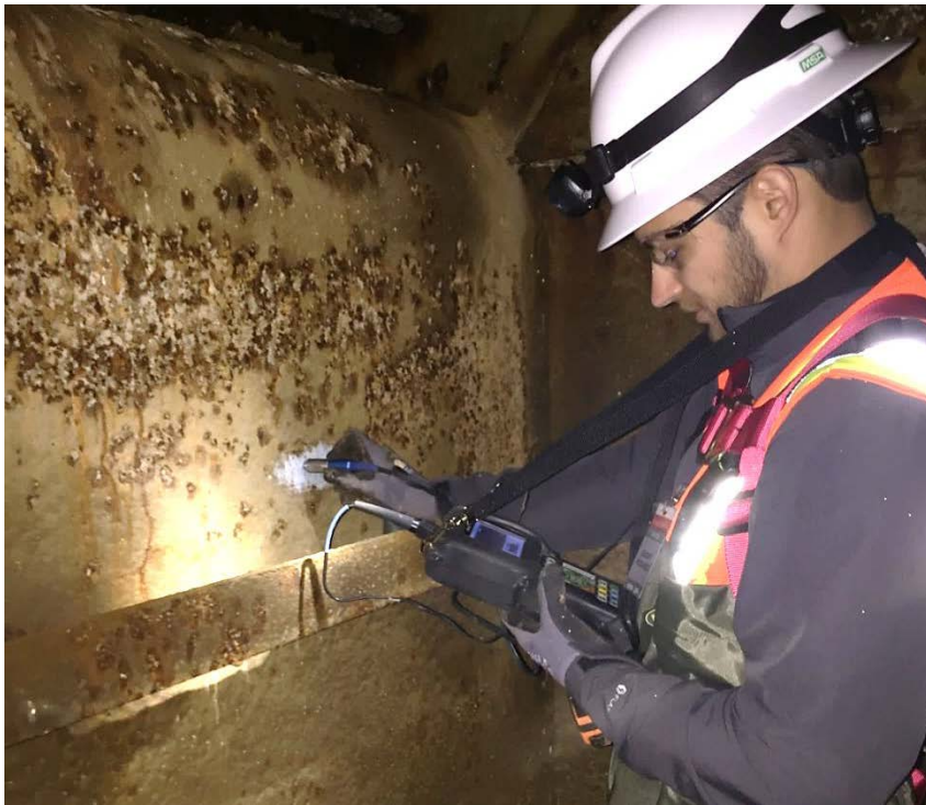
Figure 16: Process for Typical UT Measurement
