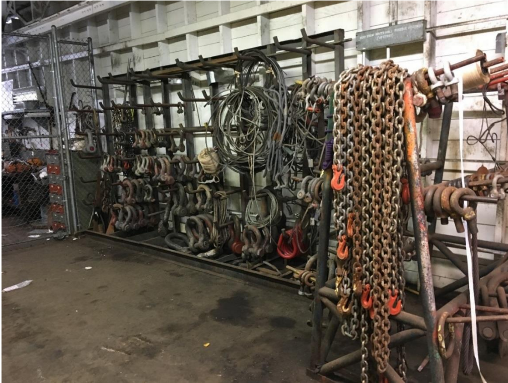
Inside Bldg. #109 (manual rigging equipment, miscellaneous sizes)
