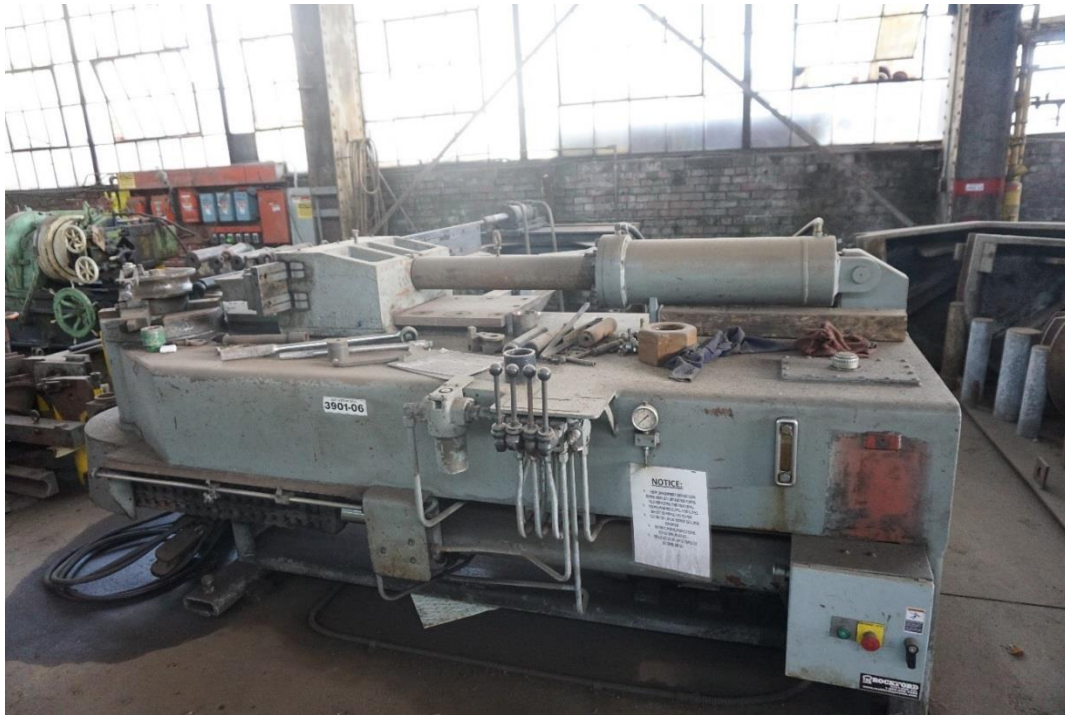
Coast 6' Iron Pipe Bender (Bldg. 105)
