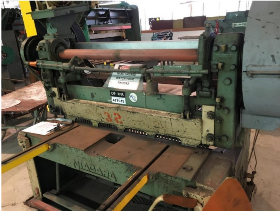
Electric Shear #32. Capacity 10 GA (Bldg. 109)
