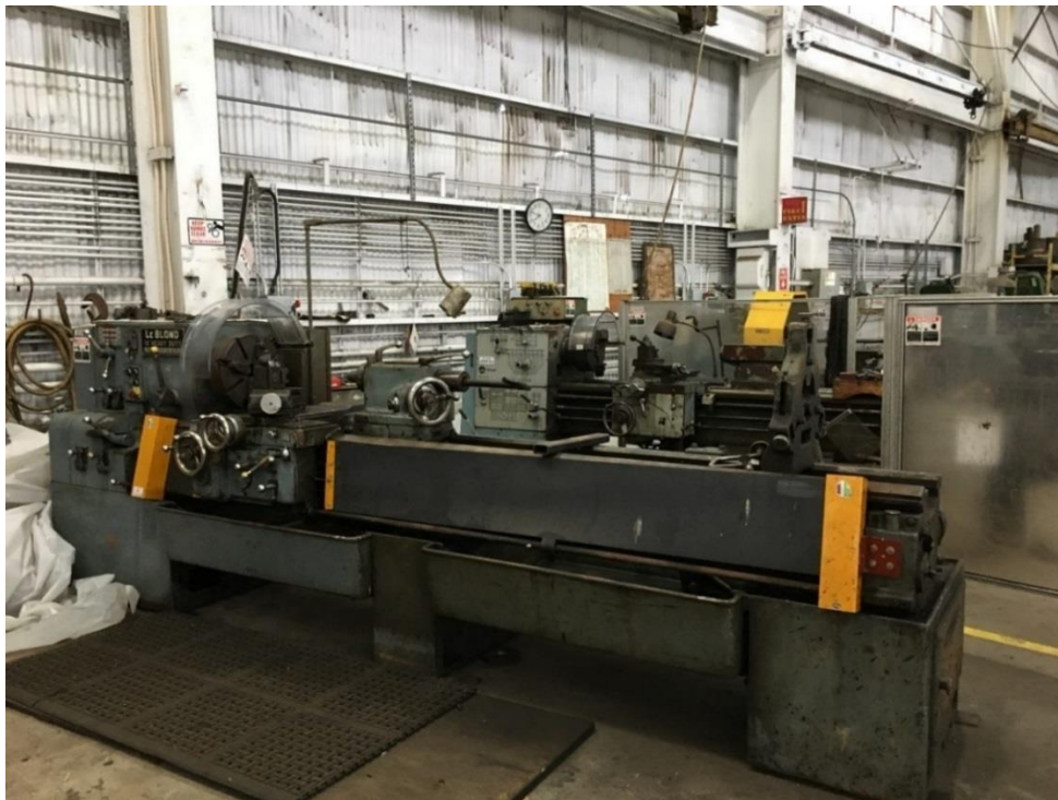
LeBlond 16-inch Heavy Duty Engine Lathe, Spindle Speed Low 16-71, med. 38-394, High 450-2000 (Bldg. 36)
