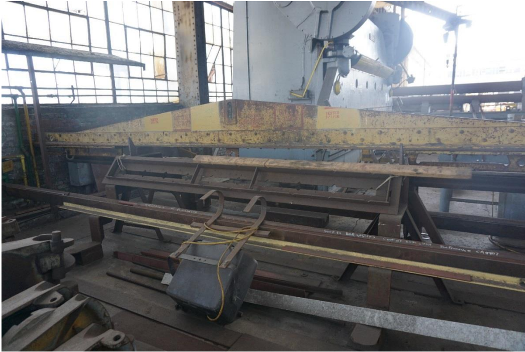
Spreader Bar 15 Ton Capacity X 15 Feet (Bldg. 105)
