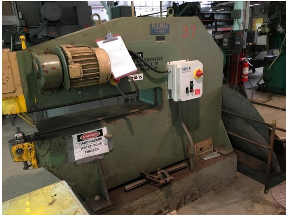
Pullmax Universal Shearing-Forming Machine #37. Capacity 10 GA (Bldg. 109)
