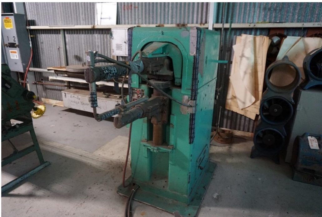
ACME Spot Welder #2 (Bldg. 109)
