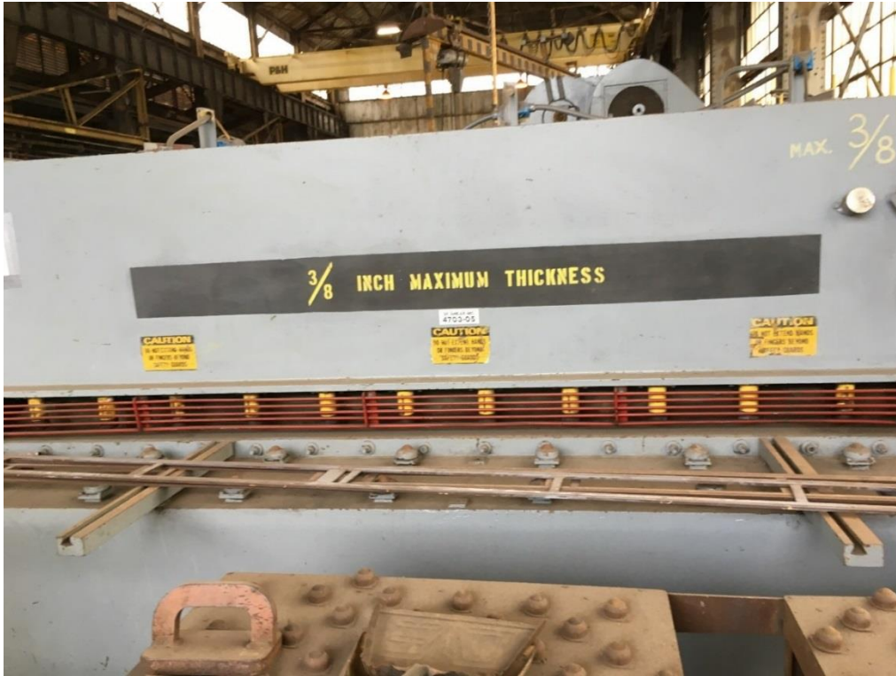
“Hydropower” 244-inch x ½-inch Shear (Bldg. 105)
