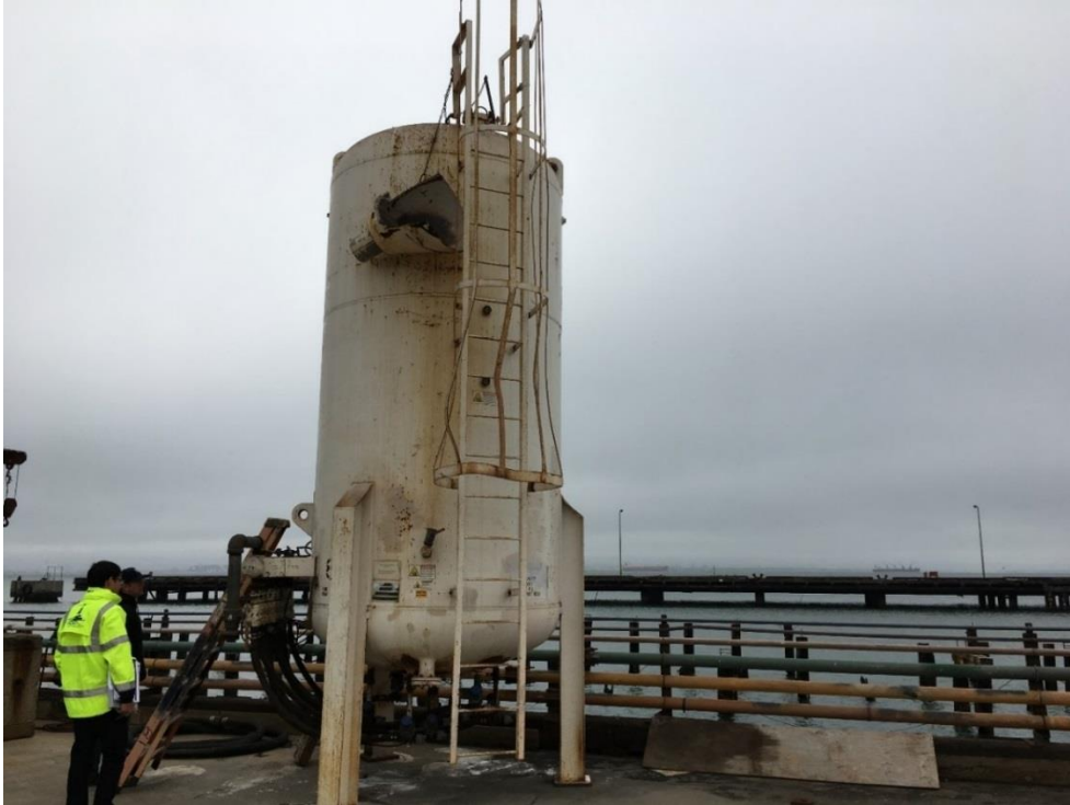
Sandblast Pot near Drydock #2 (four units – photo of typical unit shown. Tare weight=9500 lbs. each unit.)
