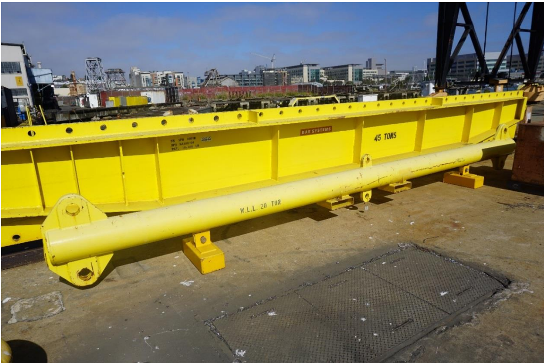
Spreader Bar 20 Ton Capacity X 21 Feet (Wharf 3)
