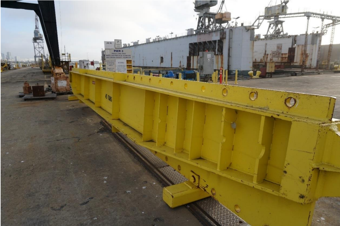
Spreader Bar 45 Ton Capacity x 36 Feet (Wharf 3)
