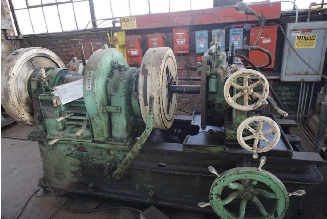
Landis 6" Pipe Threading Lathe (Bldg. 105)
