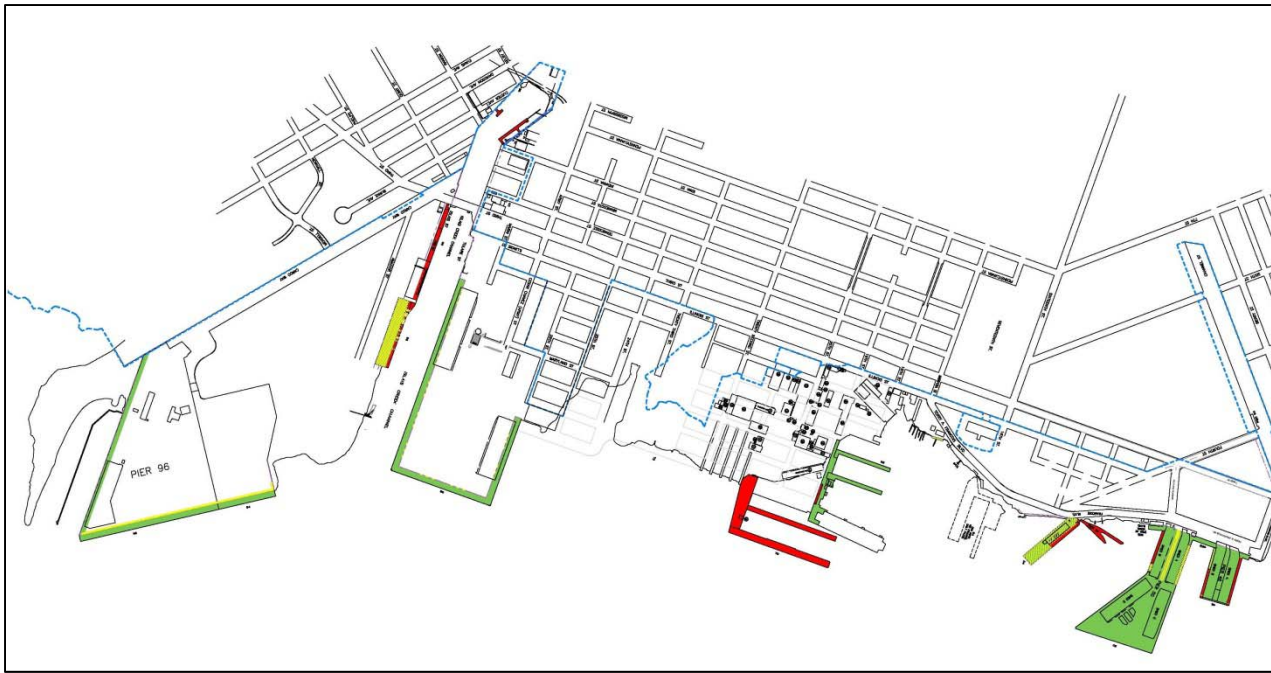
Figure 7: Structural condition rating map of substructures along the waterfront between China Basin and Pier 96
