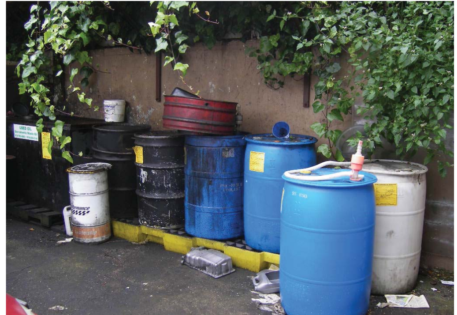
Materials are stored in bins but there is leakage, discarded oil cans, and uncovered containers.
