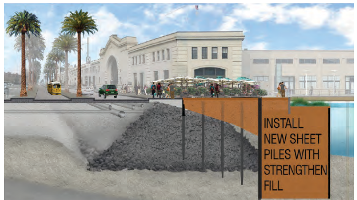
Option 3: Bulkhead Replacement
