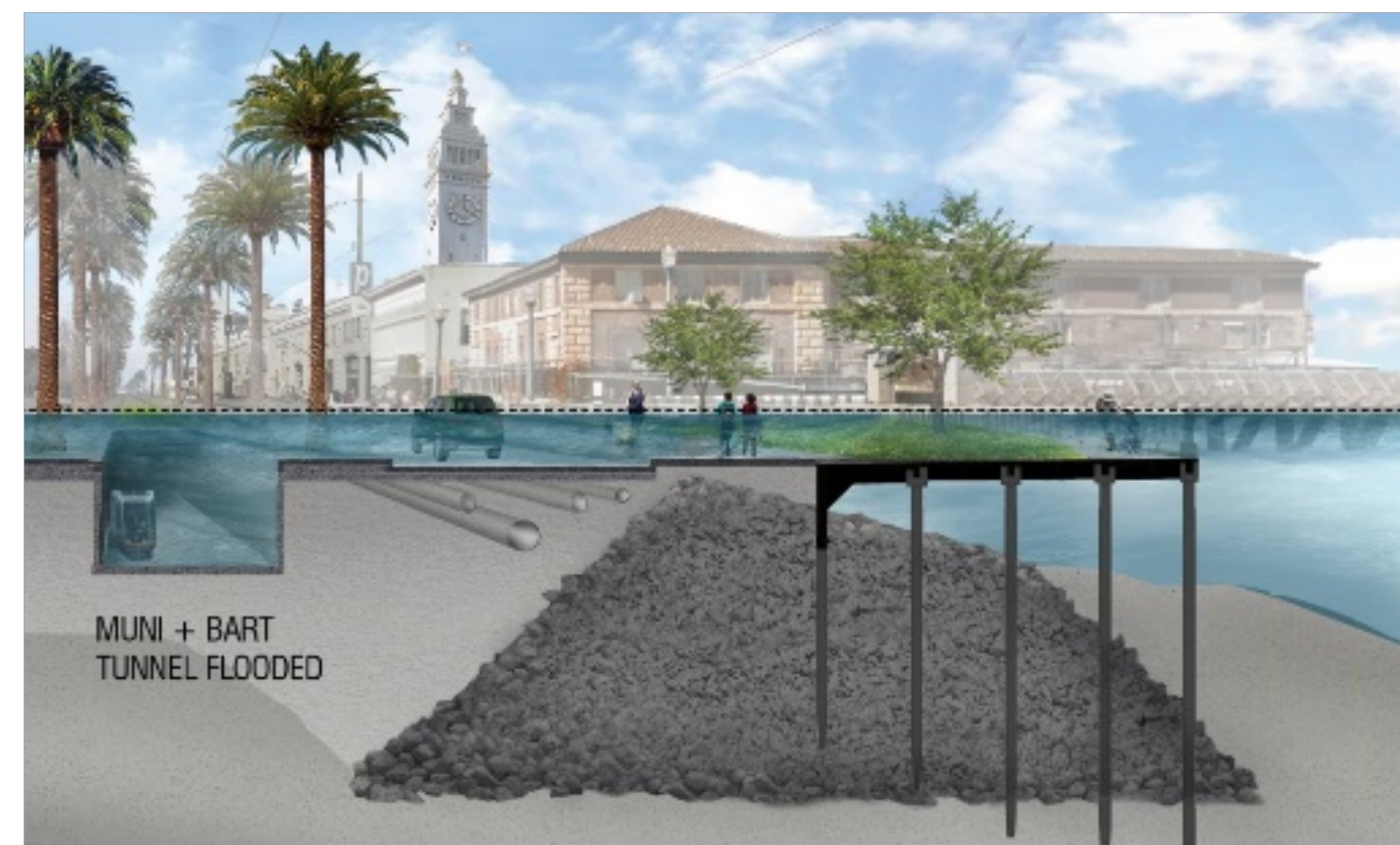
Rendering of the Embarcadero Seawall during flooding due to sea level rise.
